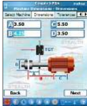
Dimensions – Enter only 4 motor dimensions for automatic shim value calculation during the alignment.
